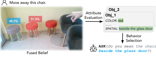
Fig. 6. Behavior Planning. Attribute-based clarification distinguishes competing targets when the grounding belief remains ambiguous.
