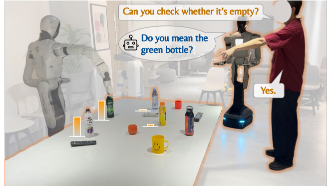
Fig. 1. MIGU fuses language cues with pointing geometry for robot manipulation under uncertainty, asking clarification questions when needed.
