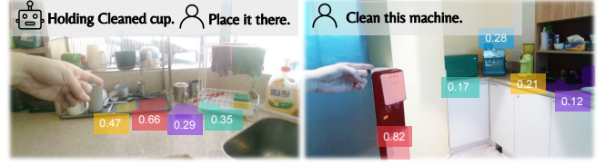
Fig. 5. Generated semantic beliefs. Left: an ideal prior. Right: a biased prior generated by the VLM.
